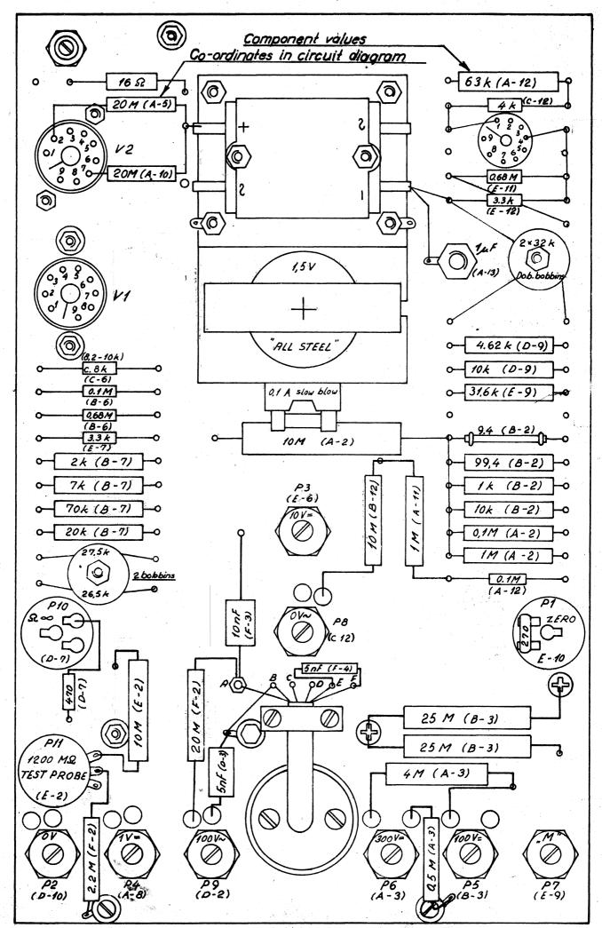
Vacuum-Tube Voltmeter, type RV23
