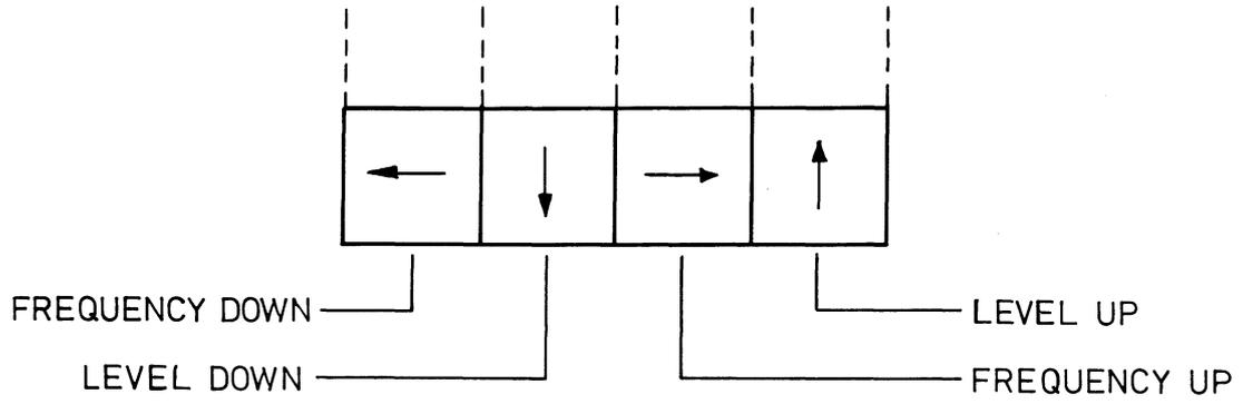
Fig. 3.17 - Level and Frequency Step Control Keys
