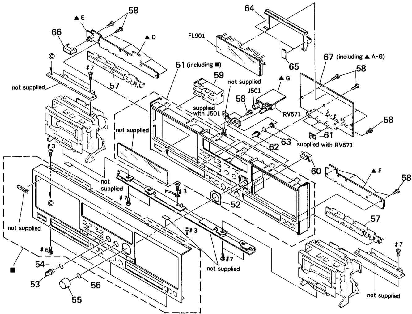
**6-3. MECHANISM DECK SECTION 1
