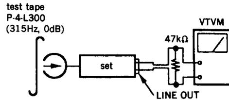
Adjust RV131 (L-CH) and RV231 (R-CH) for DECK A and RV151 (L-CH) and RV251 (R-CH) for DECK B so that the reading on VTVM meets the adjustment limits next page.
