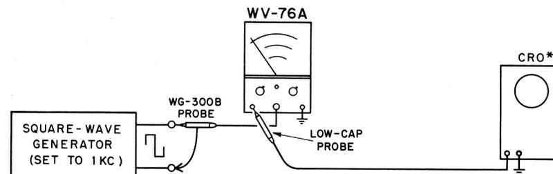
Figure 12. Test setup for frequency-compensation adjustments.
