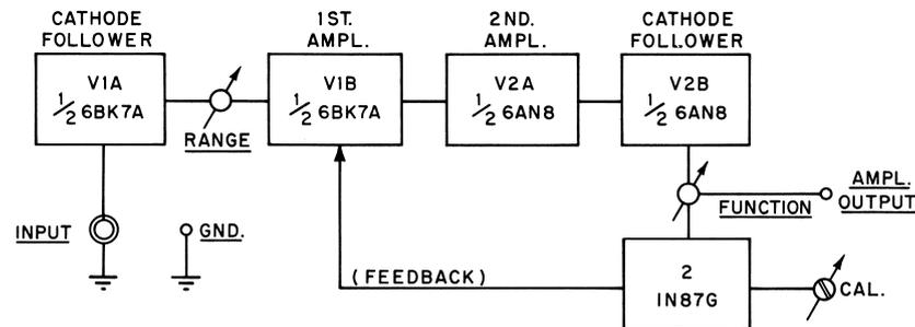
Figure 10. Block diagram of WV-76A.
