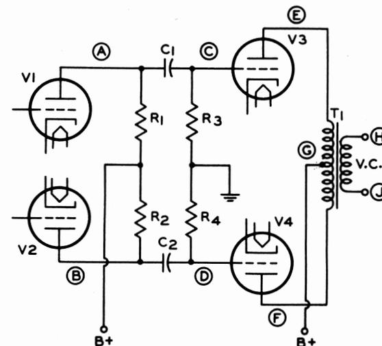
Figure 8. Test points in audio amplifier.
