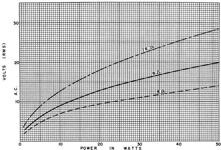
Figure 9. Graph for conversion of rms volts to power output in watts for amplifiers with output loads of 4, 8, or 16 ohms.
