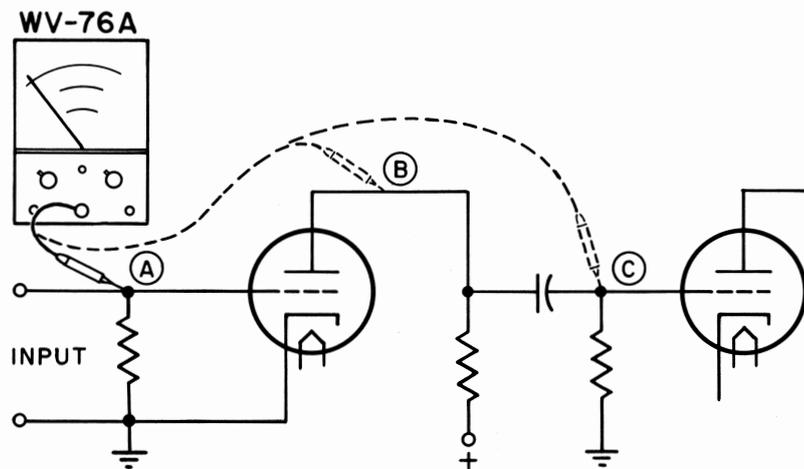
Figure 7. Test setup for voltage-gain measurements.
