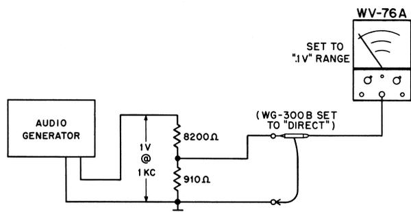
Figure 11. Test setup for voltage calibration of WV-76A.
