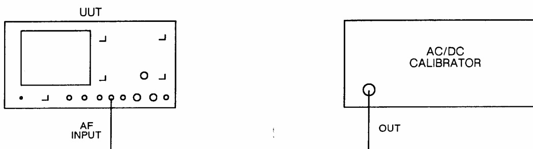
Fig. 5-1-7 Test equipment connections for voltmeter DC & AF level accuracy performance checks
