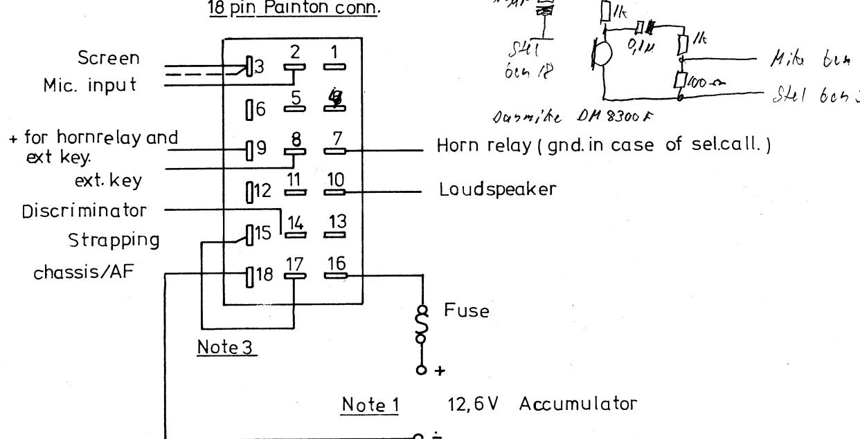
Note 1: DC converter has to be used as far as the powersupply is not 12,6VDC with chassis negative.
